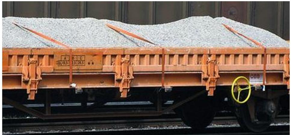
The orange panel is peeling off the tarp in this picture. Who is responsible for maintaining specification communications during transportation? Was a tarp the right choice for a durable surface to apply this marking? What can we do to prevent our markings and labels from falling off during normal conditions of transport?
