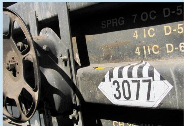
Cannot find enough flat-surface on your conveyance or package to apply your placard correctly? Are we allowed to wrap the placard around components like this on our rail cars or vehicles? Will anyone notice the hazard class is not in plain sight?
