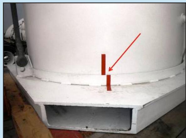
Handling and loading packages is a job for a perfectionist. This cask arrived at one of our facilities this way. Should the alignment marks line up? Was it loaded this way or did the cask shift during transportation? Either way, was the shipper at fault?
