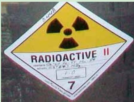
Can you identify at least 2 issues with this label? Label information must be legibly printed (manual or mechanical) using a durable weather resistant means of marking per 49 CFR 172.403(g). Maybe hard to see in this picture, but the printing in the contents and activity blocks are smudged and faded upon receipt. Also, be careful with extra information written on a label beyond what is required that may cause confusion,
