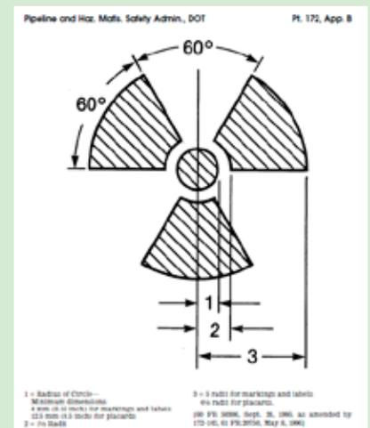
How many issues can you identify on this placard? Looking at the trefoil, does it match the allowed proportions authorized in Appendix B to 49 CFR Part 172 per 49 CFR 172.519(g)? The center dot is too big with little yellow space between the center and the blades. Also, does the package surface provide enough contrast to the placard color? If not, the placard will need either a dotted or solid line outer border to provide the needed contrast per 49 CFR 172.516(c)(7).
